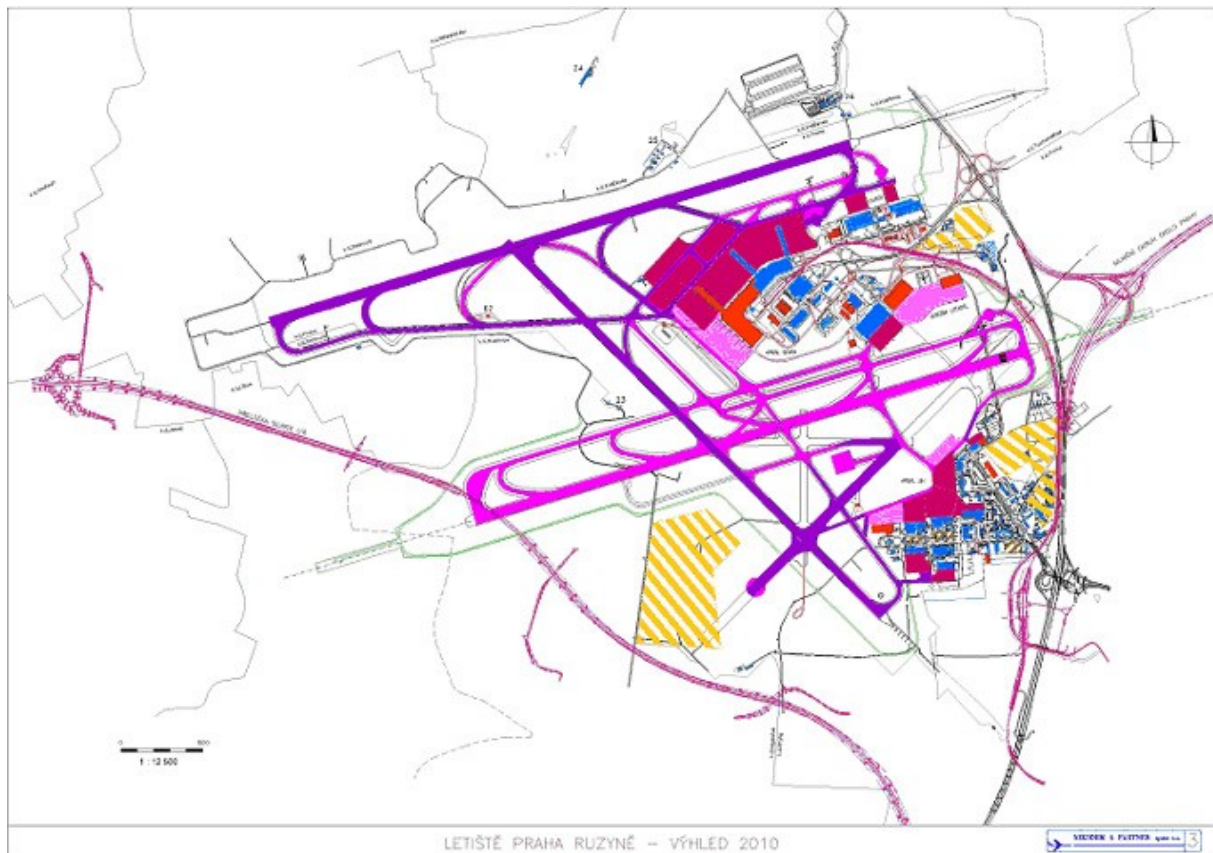
Picture no. 3 – the current Prague-Ruzynee airport runway system and the plan for construction of a new runway.
